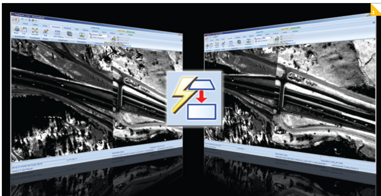
❖ FIGURE 2 The Ortho On-the-Fly tool streamlines geospatial production while improving accuracy and reducing geometrical measurement errors associated with sensor and terrain modeling. It orthorectifies (stitches together) raw images in real time to produce a continuous, highly accurate image of an expansive area, allowing first responders and analysts in the field to view and analyze imagery without delay.
