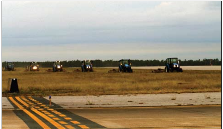
The flightline at Eglin Air Force Base, Fla., is nearly 75 percent safer than years previous because of improvements to its Bird and Wildlife Aircraft Strike Hazard, or BASH, program. One of the changes was to keep the grass height higher around the runways because birds are less likely to land somewhere if they can't see each other. [Photo courtesy of U.S. Air Force]
