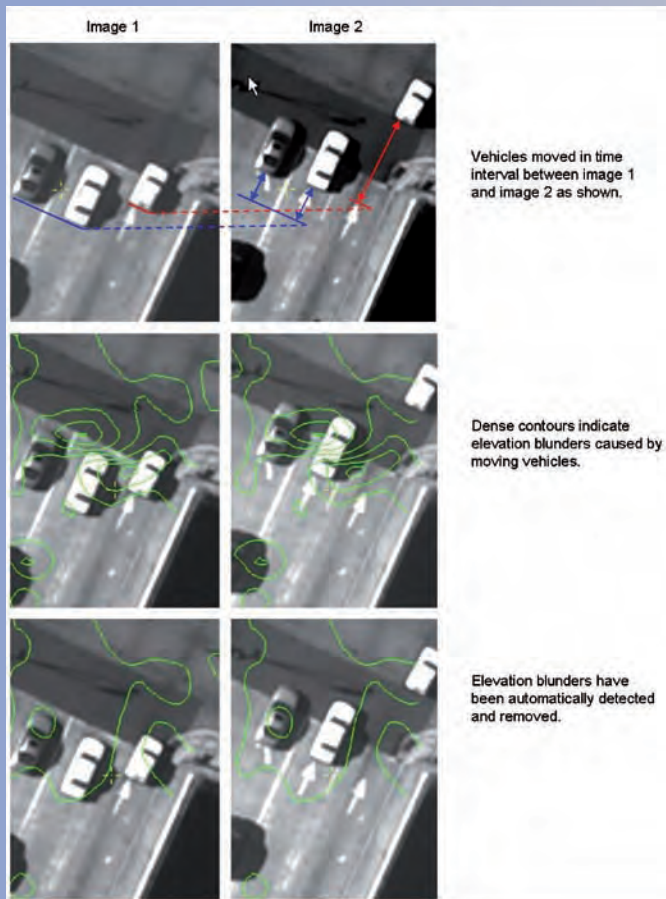
Figure 1. Moving vehicles cause three false matches on the middle images. The three false matches result in elevation blunders. Note how in the lower images, the algorithm has detected and removed the blunders.
