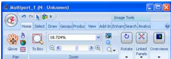
The Ribbon scales to accommodate screen size; on smaller displays space is economized by hiding labels, replacing large icons with small ones, and consolidating functional groups.
